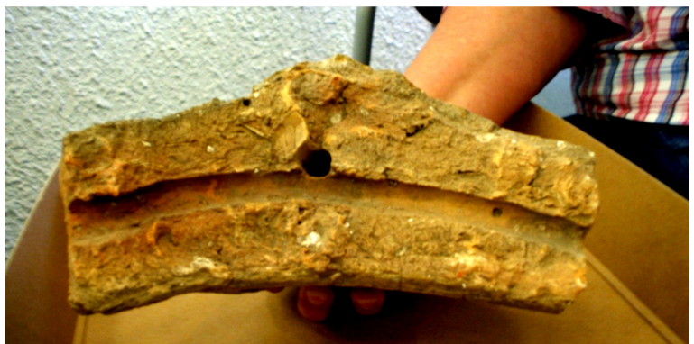
Fire-bar showing method of construction
